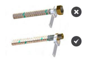
FIGURE 14: ACCOUNTING FOR SHRINKAGE IN FLEX HOSE
